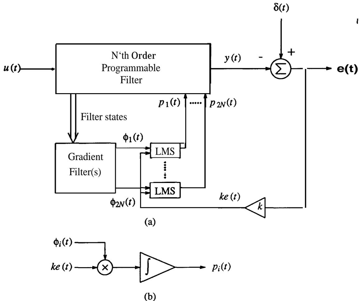
Fig. 3. Block diagram of a LMS gradient adaptive filter.
