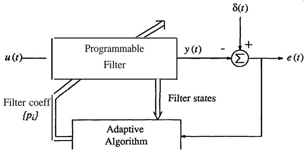
Fig. 1. Block diagram of an adaptive filter.
